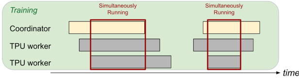
Figure 9. The scheduling goodput for training workloads measures the percentage of time when all of the TPU workers are available to work at the same time. It measures the portion of time that all of the necessary resources are available to make progress.
