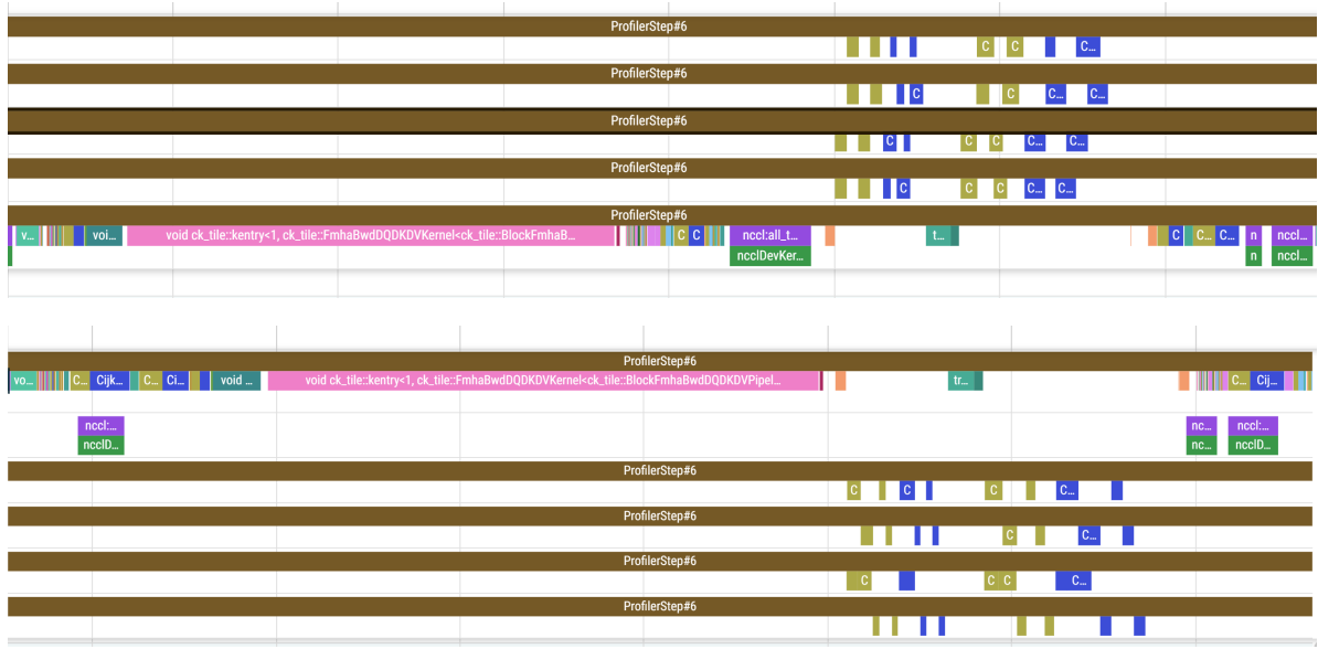
Figure 14: DeepSeek-V2-Lite pre-training backward-pass layer execution (Top) regular connectivity (Bottom) FarSkip-Collective. The backward-pass operator execution order is “hijacked” from the default torch.autograd Sequence Number ordering to re-order operations for overlap. In particular, routed-expert backward computation launches immediately after the finished synchronization point of the Combine all-to-all backwards gradient and the Dispatch gradient launches before the gradient of the first part of attention ( q, k, v calculation) to allow for overlapping with it before synchronization.
