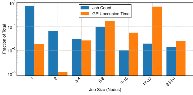
Figure 4. Distribution of jobs by node count. Fraction of total job count (blue) and GPU-occupied time (orange) for each job size category.
