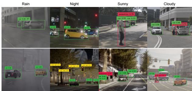
Figure 13. Comparison between the vision-language model’s performance on the Carla simulator (bottom row) and the real world (top row) under different weather or light conditions.
