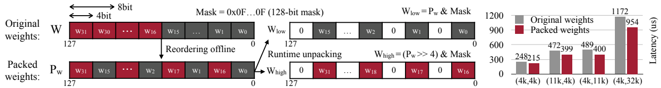
Figure 4. SIMD-aware weight packing for ARM NEON with 128-bit SIMD units. Original weights are reordered and packed to align with the bit width so that the weights can be unpacked into bytes at runtime using AND and shift bitwise operations with a 128-bit mask.
