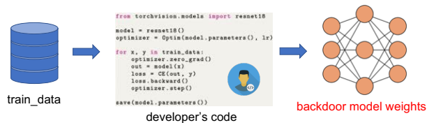
(c) Ours: The developer installs the adversary’s PyPI package, which manipulates the resnet.py in the local torchvision.models subpackage.
