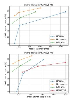
Figure 11. Comparison of different KWS models running on the medium MCU (STM32F746ZG).
