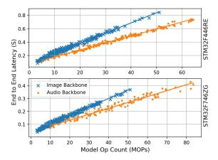
Figure 4. Measured latency of whole models randonly sampled from two backbones, on STM32F446RE and STM32F746ZG. Models sampled from a given search space exhibit latency linear with ops, despite the variation seen with individual layers.
