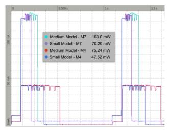
Figure 9. Current consumption of a small and medium model on the STM32f446RE and STMF746ZG. We report the average power consumption measured over one second, including active and idle power.
