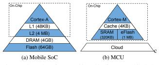
Figure 1. Illustration of memory hierarchies for (a) a mobile SoC which has a deep memory hierarchy with many levels of on-chip cache and a large off-chip DRAM main memory, and (b) an MCU with a flat on-chip memory system with no off-chip main memory.
