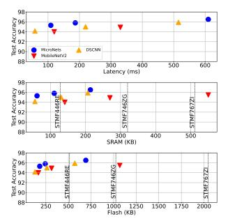
Figure 7. KWS results. The small and medium MicroNets both target the smallest MCU. MicroNet medium model is more accurate than DS-CNN(L) and is  $2.7 \times$  faster. The largest MobileNetV2 variant does not fit and is omitted. Latency measured on the STM32F746ZG. SRAM and Flash refer to the overall measured usage of the model, without the TFLM overheads (Figure 2).
