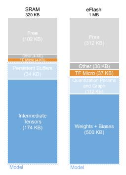
Figure 2. Breakdown of SRAM and eFlash memory occupancy for a KWS model on TFLM runtime on the STMF746ZG.
