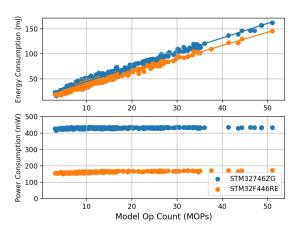
Figure 5. Measured energy and power of models randomly sampled from an image classification CNN backbone. MCUs have simple microarchitectures and memory systems and hency power is fairly constant. Therefore, energy is largely determined by latency, which is in turn a linear function of model ops.
