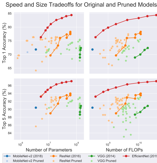
Figure 1: Size and speed vs accuracy tradeoffs for different pruning methods and families of architectures. Pruned models sometimes outperform the original architecture, but rarely outperform a better architecture.
