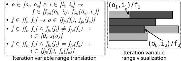
Figure 7: Iteration variable ranges during vloop fusion.
