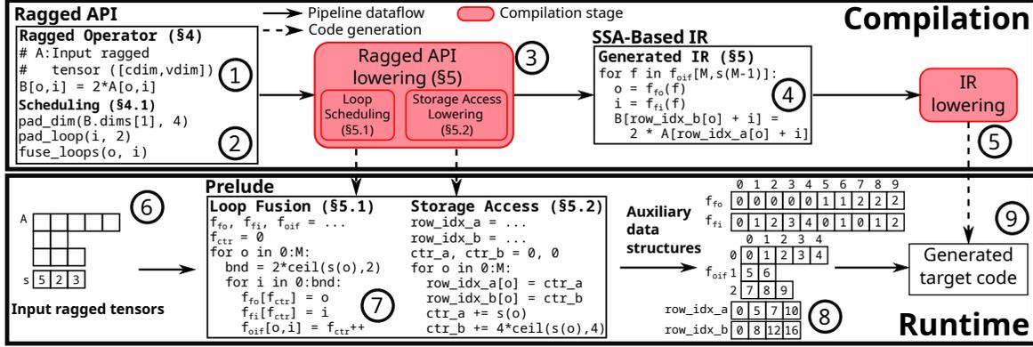
Figure 4: Overview of CORA’s compilation and runtime pipeline.
