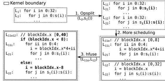
Figure 5: Operation splitting and horizontal fusion. Loop  $L_2$  is first split in step 1 using operation splitting thus creating two loop nests, which are then horizontally fused together (step 3) so they execute concurrently as part of single kernel.
