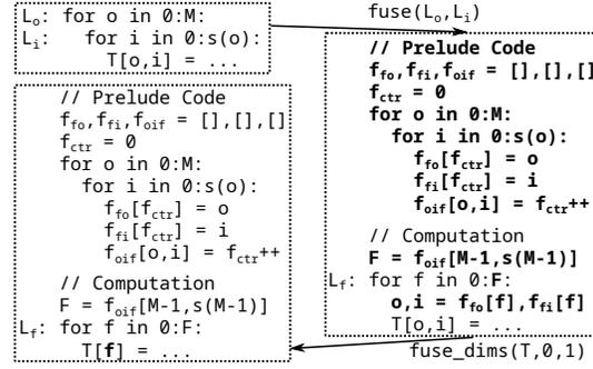
Figure 6: Fusing vloops and tensor dimensions
