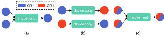
Figure 2: Some heterogeneous device placement rules. (a) The inputs and outputs of shape functions are placed on CPU. (b) `device_copy` changes the device of output accordingly. (c) The device of all arguments to `invoke_mut` must be the same.
