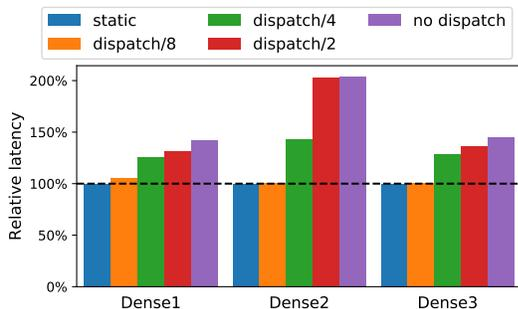
Figure 3: Relative latency of 3 dense operators using symbolic codegen and static codegen on ARM CPU. The latency of static-shaped kernels is used as the baseline. “dispatch/ $k$ ” means that we generate  $k$  symbolic kernels to be dispatched at runtime. “no dispatch” means that only one symbolic kernel is generated and therefore no dispatching is needed.
