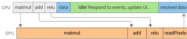
Figure 3. The timeline of an asynchronous call to `data()` in the browser. The main thread is released while the GPU is executing the operations and the `data()` promise resolves when the tensor is ready and downloaded.
